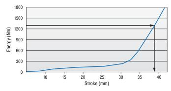
Force stroke characteristic curve (dynamic) (With impact velocity range over 0.5 m/s)
