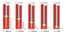
\* The load velocity reduces continuously as you travel through the stroke due to the reduction in the number of metering orifices (\*) in action. The internal pressure remains essentially constant and thus the Force vs. stroke curve remains linear.
