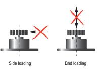
Note! The rotary axes, square mounts or free-wheel mounts are not designed for side loading.
